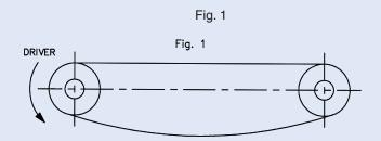
**Setup:** Horizontal; slack lower strand. **Problem:** Normal chain wear causes loss of tension.
