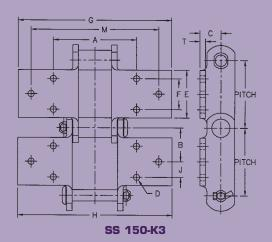
**DIMENSIONS IN DECIMAL INCHES** AVERAGE D MOLINE WEIGHT ATTACHMENT BOLT HOLE PER FT. PITCH LBS. NO. C DIAMETER DIAMETER Ε F G A В Н J М Ν Т 6.56 1.88 0.50 0.56 4.25 2.75 13.50 13.56 1.38 0.50 27.3 SS 856-K3 6.000 3.00 10.94 12.06 SS 150+-K3 6.050 7.50 3.02 1.88 0.50 0.56 4.25 2.75 13.81 13.88 1.38 11.50 0.50 26.9
