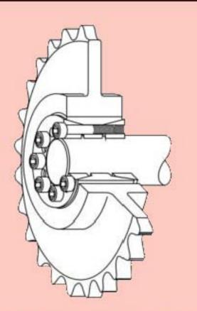
Keyless Lodding Devices provide heavy duty, worry-free connections for all types of sprockets ...
