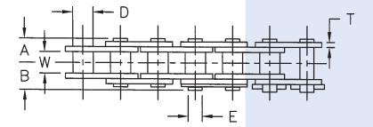
Plated roller chain is standard chain which is nickel-plated before assembly. It features a sheen and has the property of being resistant to corrosion, together with almost the same strength and wear resistance as standard roller chain.
