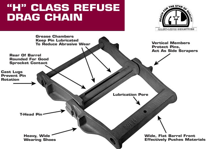
Moline Refuse Drag Chain is used for conveying sawdust, wood chips, pulp, garbage, tankage, ashes, and other abrasive waste materials through either wooden or steel troughs. Because of its large, wide opening area, Moline Refuse Drag Chain provides sizeable carrying capacity when operated at moderate speeds.
