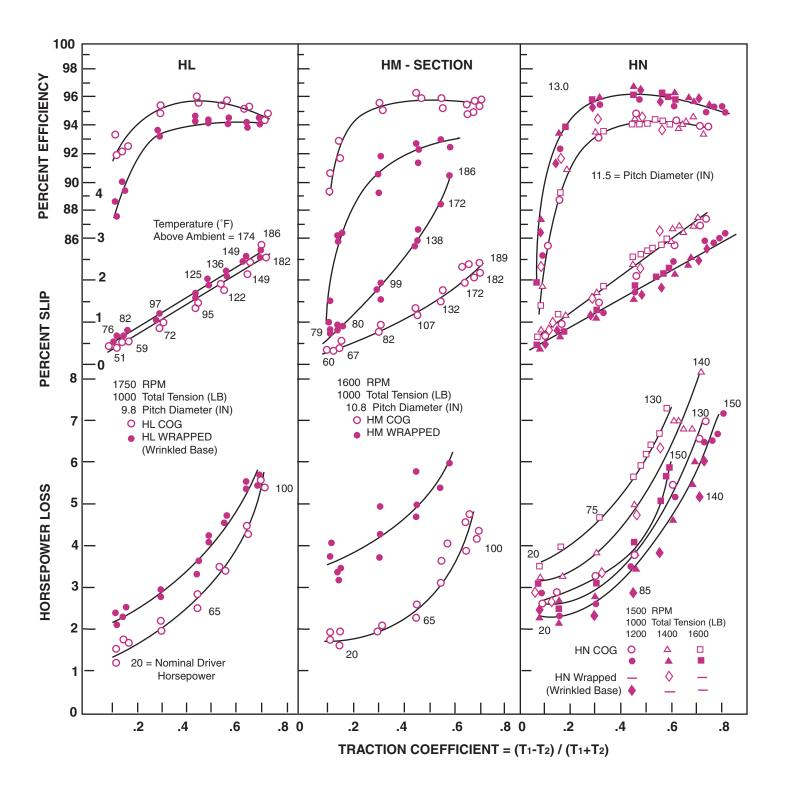
Fig.6 Agricultural variable speed belt efficiency, slip, temperature, and power loss
