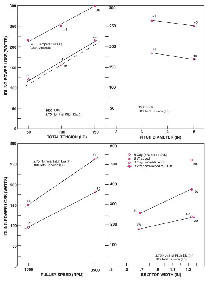
Fig. 3 Idling Power Loss Dependence on Tension, Diameter, Speed and Width
