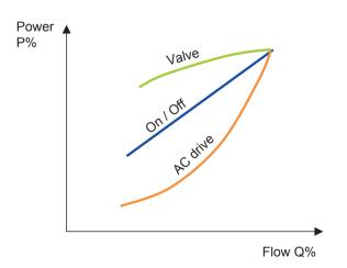
Electrical power consumed by pump at partial loads is remarkably less than with on/off or valve control.
