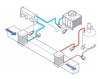
The basic building blocks of an HVAC system: chilled water circulation, hot water circulation and air circulation.
